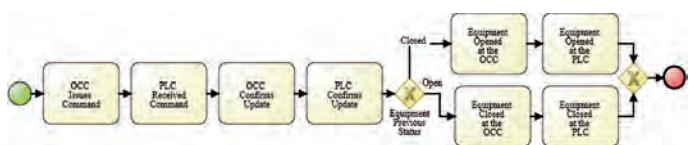
BP-IDS detecting injection of a command at a PLC. © INOV
